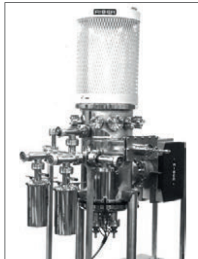
1971 Conventional joule-effect evaporator with glass hood.
